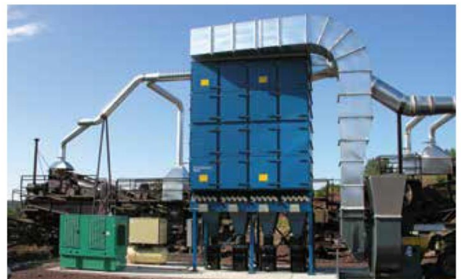
DLMC on Rock Crushing 41,000 cfm (69,645 m 3 /h)
