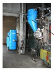
The 1020MFS shown to the left is being used to reclaim Steel Shot and introduce it back into the customer's shot blast machine via a 'VAC-U-MAX Intercept Hopper.
