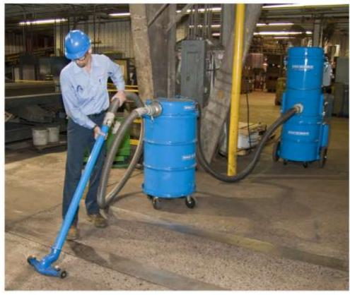
The 1020MFS is typically used with a material intercept: either a 55-gallon drum, or a forkliftable self-dumping hopper. The 55-gallon drum will allow access to confined areas, while a 1or 2 cubic yard hopper will offer up to 50 cubic feet of collection capacity.
